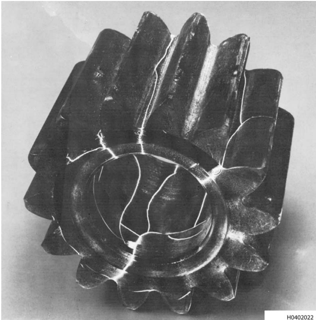
Figure 3-41. Typical Magnetic Particle Indications of Cracks
