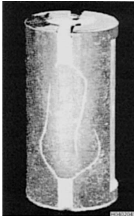
Figure 3-60. Magnetic Particle Indications of Quenching Cracks Shown With Dry Powder
