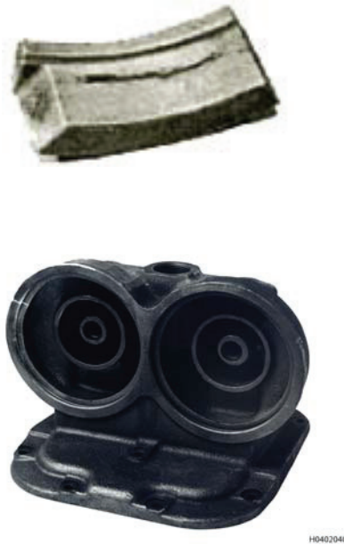
Figure 3-59. Magnetic Particle Indications of Defects in Castings
